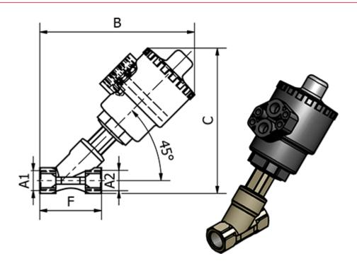
B = 270 C = 264 Connecting A1 = G 1 1/2" Connecting A2 = G 1 1/2" Control Air = G 1/8" Control Air = 4-8 bar F = 120 Max. Working Pressure = 11 bar
